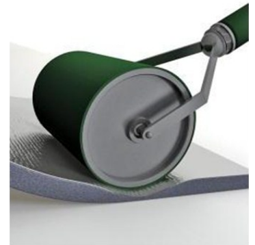
Thicker PSA products are best rolled
