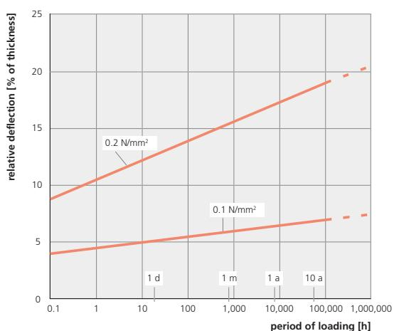
increase in deformation under consistent loading
