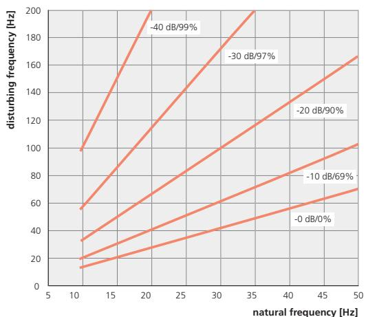
reduction of the transmitted mechanical vibrations by implementation of an elastic bearing consisting of Sylomer P
