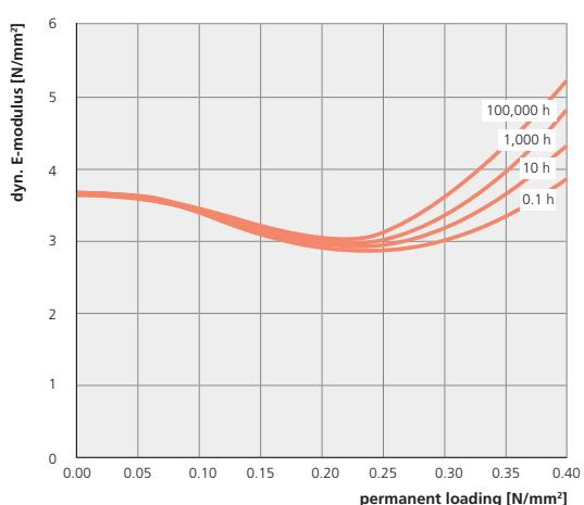
change of dynamic modulus of elasticity under consistent loading
