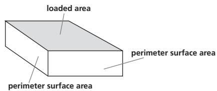
The shape factor has an influence on the deflection and the static load limit respectively.
